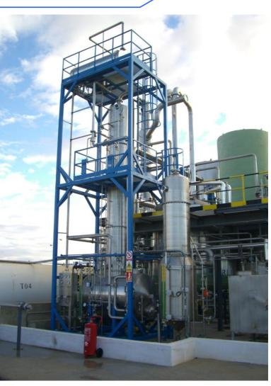
Specially designed for processes where methanol has a graduation over 85%
