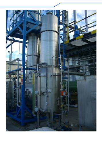
Over 99,5% purity is reached from an impure fatty acid methyl ester (FAME) coming from the biodiesel fabrication process
