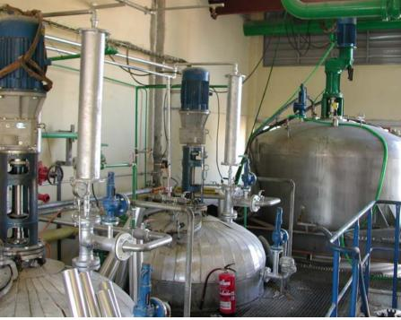
Variable stirring speed design, full control of the biodiesel reactions through a computer software
